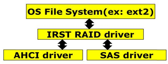
There is an option ROM (OROM) component in the BIOS that can create Intel RST RAID volumes and serves as the interface to the Intel RST RAID volumes in the preboot environment. Before the BIOS passes control to the system bootloader, the OROM leaves a copy of the features it supports, such as RAID 5, in system memory. This data can be read by mdadm to determine what features can be used when creating an Intel RST volume.
