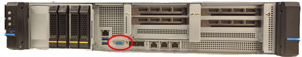
Picture depicted the connector of VGA D-Sub 9. VGA output in Front Panel
