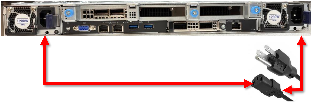
Picture depicted how to plug in the PSU cable
