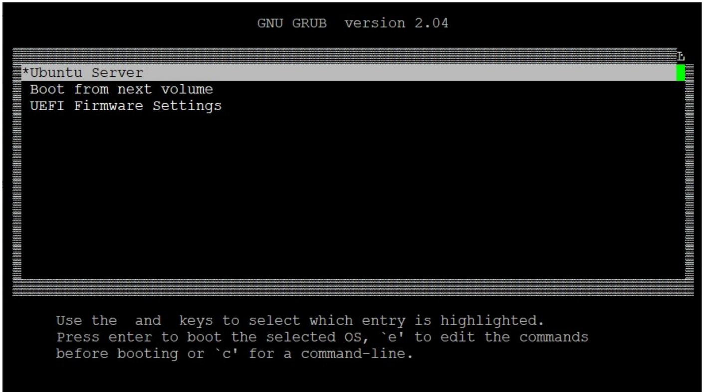
Add “console=ttyS0,115200” in grub setting, and Press Ctrl-x or F10 to boot in Ubuntu 21
