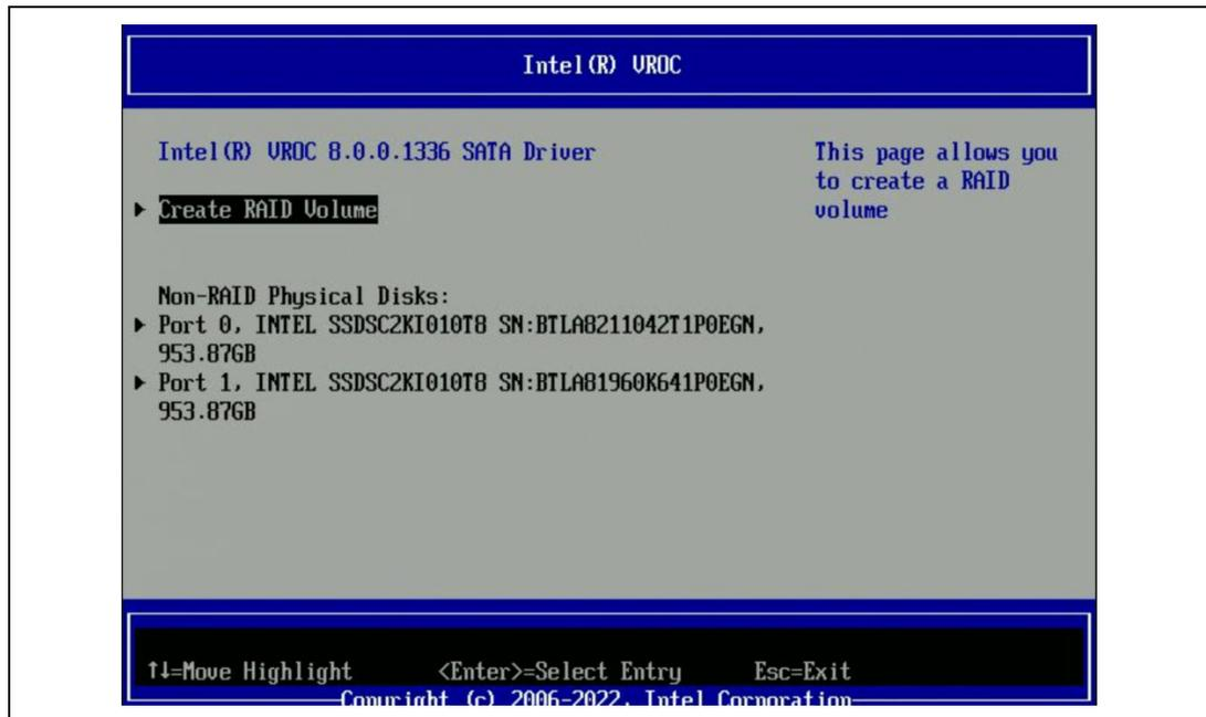
4. Press the <Enter> key to type in a volume name or move down the cursor to accept the default name.
