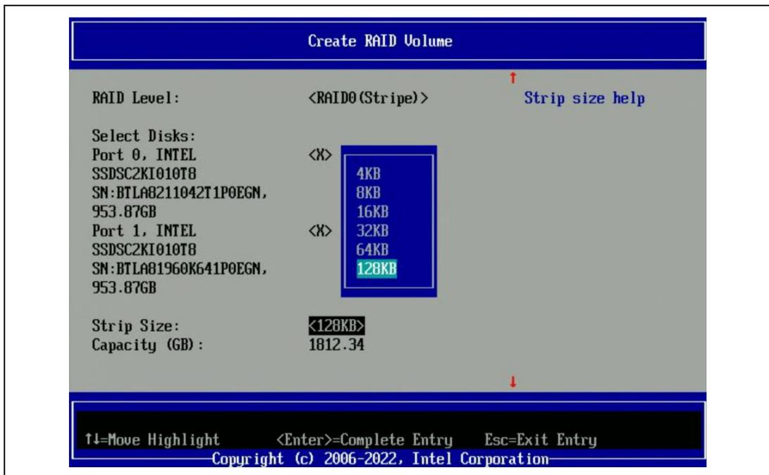
9. Select the volume capacity and press the <Enter> key. The default value will be displayed as the maximum capacity available with the drives selected. The value is calculated in bytes. A 700GB drive would use the following math:  $700 * 1024 = 716000$ .
