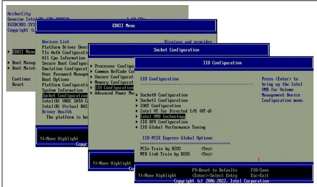
6. Using the arrow keys, move the cursor to **Intel VMD for Volume Management Device on Socket 0** and press <Enter>.
