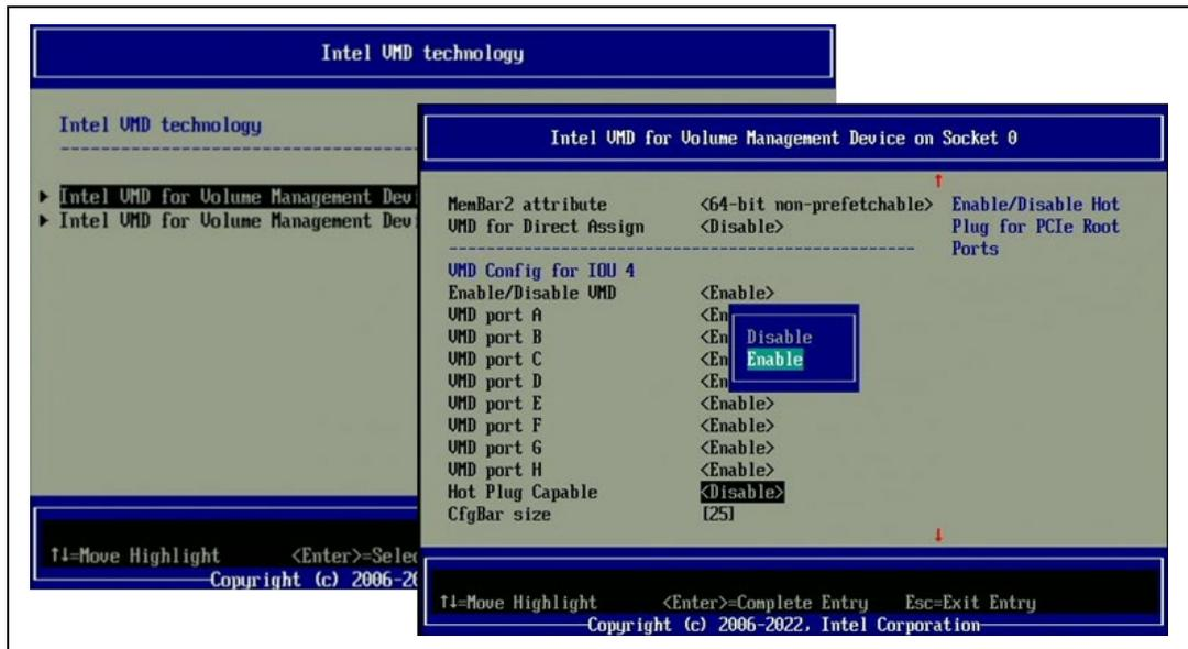
8. Press <Esc> and then move to **Intel VMD for Volume Management Device on Socket 1**. Do the same enabling of VMD functions on the corresponding IOU# ports. In this example, IOU 0 is enabled with VMD function on all the A-H ports.
