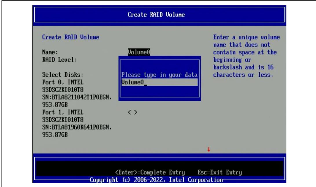
5. Select the RAID level by pressing the <Enter> key and using the arrow keys to scroll through the available values. Highlight the desired RAID type and press <Enter> to set the RAID type.
