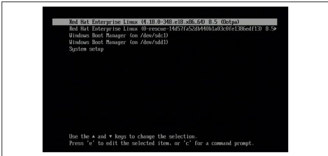
10. Add `initcall_blacklist=vmd_drv_init` in the Linux\* boot command line, and then press `Ctrl + X` to start.
