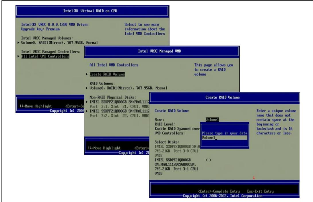
6. Press the <Enter> key, then select the **RAID level** by pressing the <Enter> key and using the arrow keys to scroll through the available values. Highlight the desired RAID level and press <Enter> to set the RAID level.
