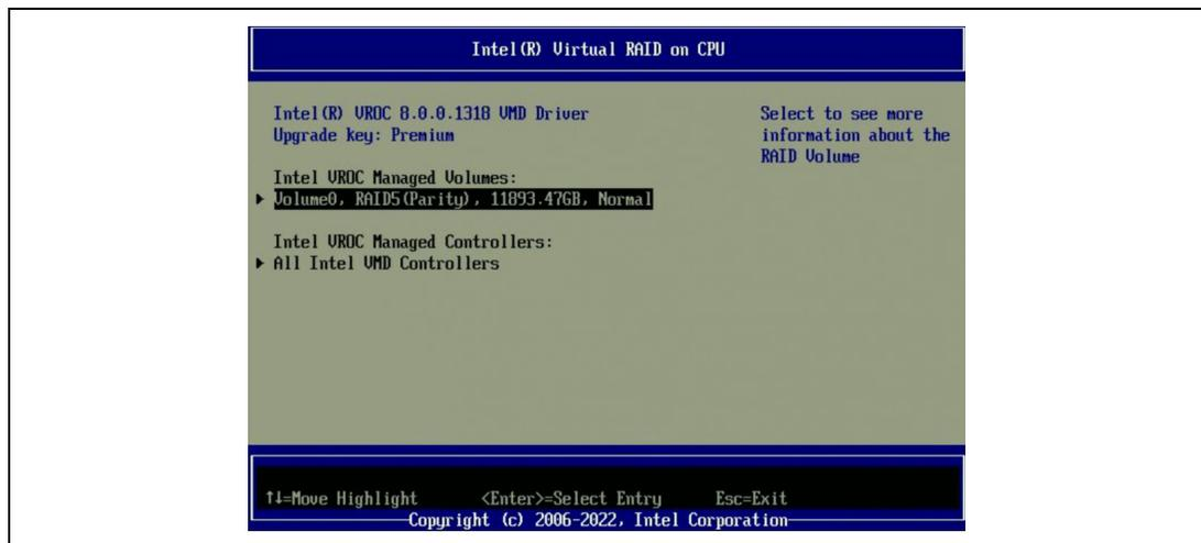
5. Navigate to **Delete** and press <Enter>, select **Yes** and press <Enter> to confirm the removal of the RAID volume.
