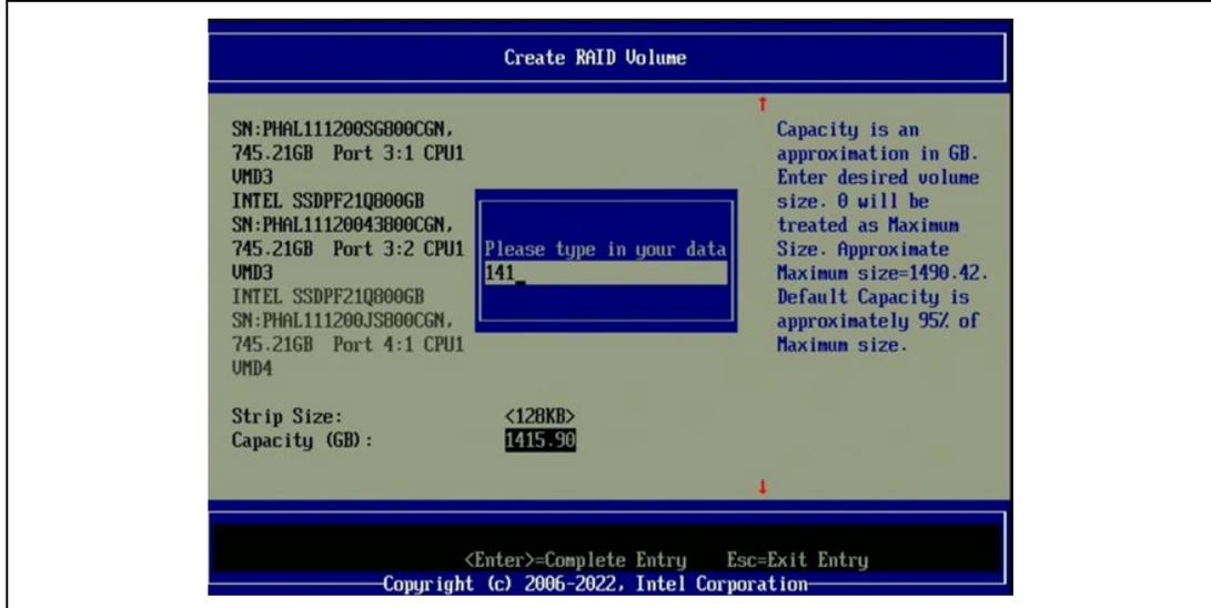
12. Navigate to **Create Volume** and press <Enter>. When showing the warning, select **Yes** to create the RAID volume.
