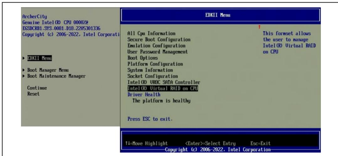
4. Navigate to **ALL Intel VMD Controllers** and press <Enter>, then select **Create RAID Volume** and press <Enter>.
