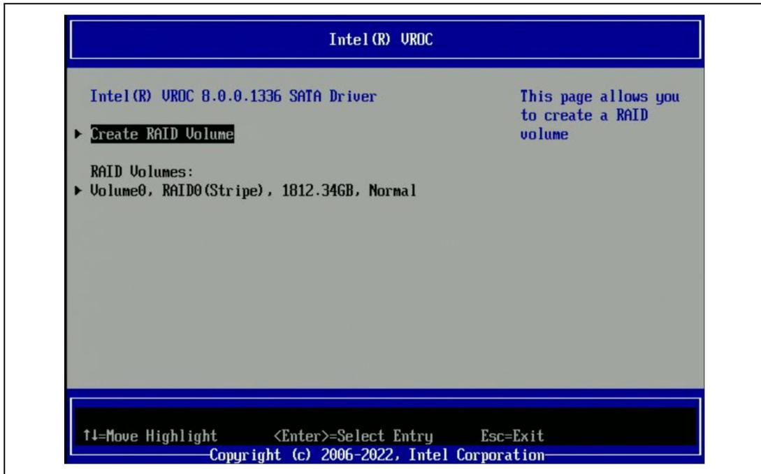
12. To exit the user interface, press <Esc>. Press <Esc> again, the user will be presented with the following message: "Changes have not saved. Save changes and exit? Press 'Y' to save and exit, 'N' to discard and exit, 'ESC' to cancel". Press <Y> to save and exit.
