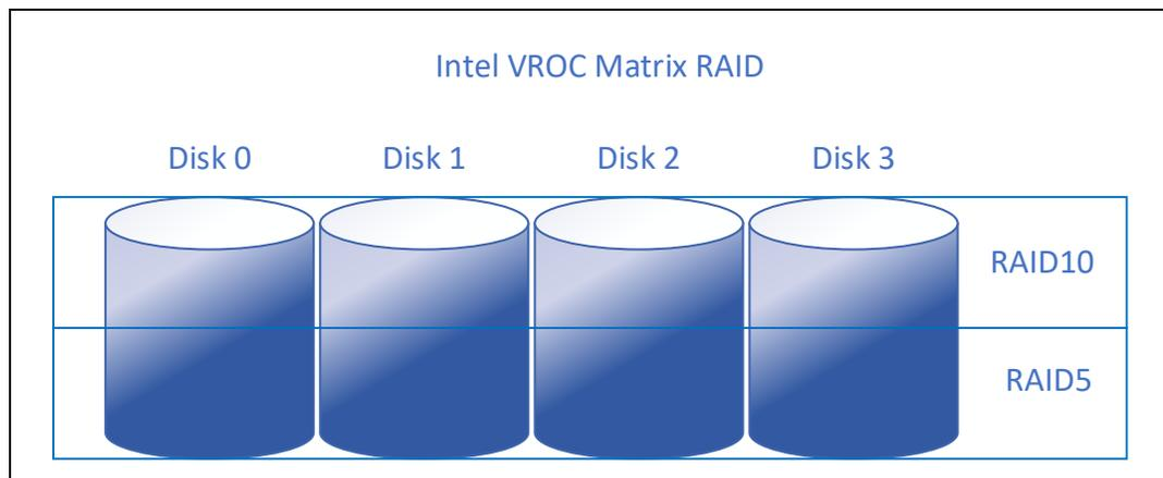
As an example, in the above diagram, on an Intel® VROC enabled system, Intel® VROC Matrix RAID allows you to create both a RAID 10 volume as well as a RAID 5 volume across four drives. Refer to [Section 4.2.5 Additional INTEL® VROC RAID Volume Creation Examples](#) to learn how to create Intel® Matrix RAID.
