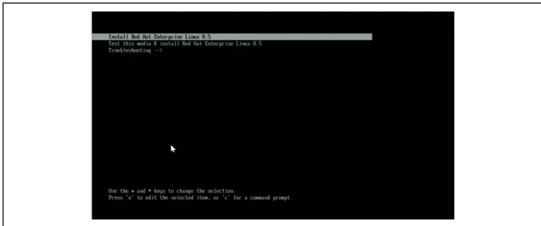
3. Add `inst.dd initcall_blacklist=vmd_drv_init` to the end of the kernel boot command line. Press Ctrl + X to continue with the installation.
