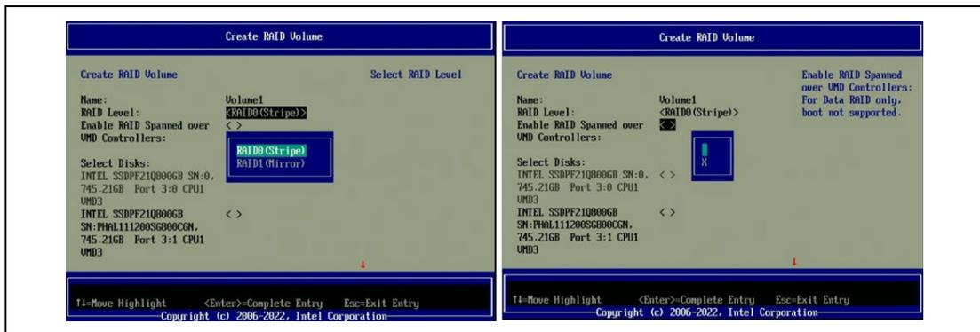
8. Press the <Enter> key. Using the arrow keys, select the drives one by one by highlighting the < > bracket on the line next to the drive's port number. Press <Enter> to open the selection menu which will be set to blank or off status. Navigate to highlight the X and press <Enter> to include the drive within the array.
