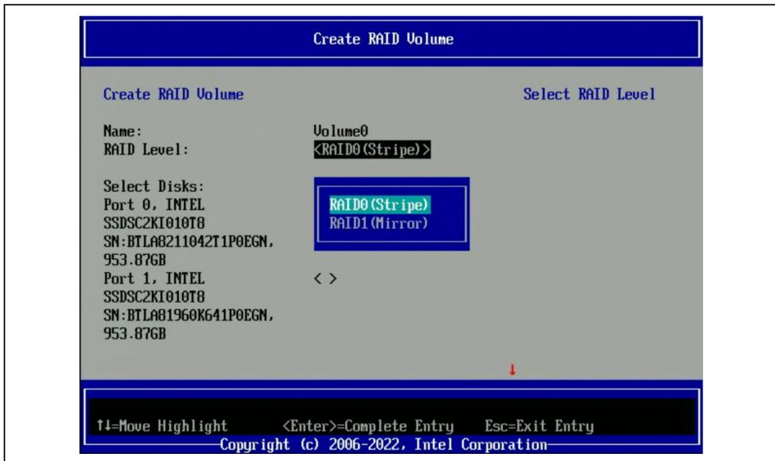
6. Using the arrow keys, select the drives one by one by highlighting the < > bracket on the line next to the drive's port number. Press <Enter> to open the selection menu, which will be set to blank or off status. Navigate to highlight the X and press <Enter> to include that drive within the array.
