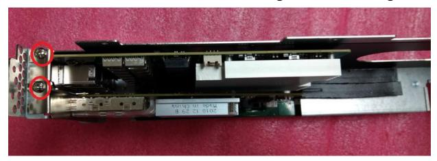
2. Please install cage's screws with a screwdriver
