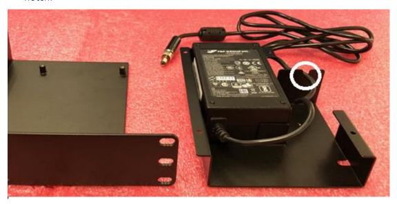
Please use 4 screws to fix PSU cover and "RMT right side kit", Power LED needs to put upper side, and tied up the Adapter cable.
