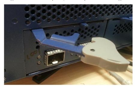
3. Please close NMC latch in system, it finishes Latch type NMC module installation.
