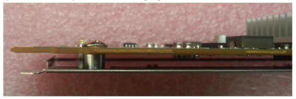
4. When Thumb-screw type NNC installation is finish, please lock 2 Thumb-screws & fixed screw.
