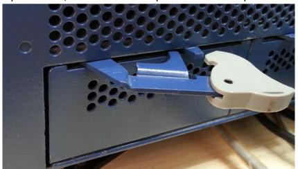
2. Please install Latch type NMC module in system, it can easy to install Latch type NMC in system.
