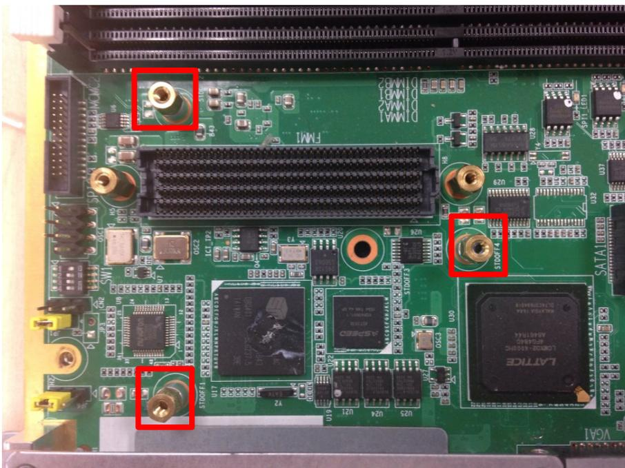
Note: Those 3 copper pillars must be removed before install FMM or FMM may get electrical damaged. (请注意上图红框处三个铜柱一定要移除，否则配合 FMM 使用时会有短路烧毁板卡的风险)
