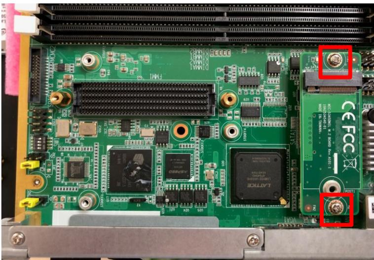
5. Remove FMM front panel, then you can install FMM(移除前挡板即可装上 FMM 模块)
