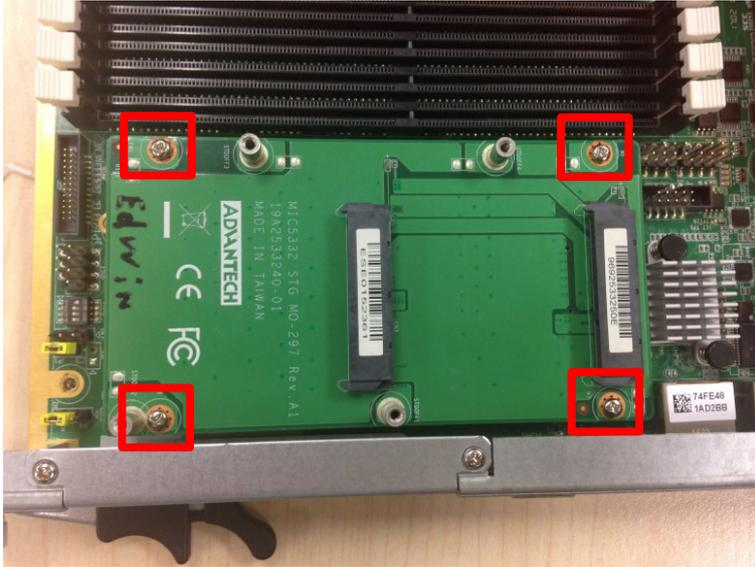
2. Remove 3 copper pillars as following red marked (卸除上图黄框的四颗螺丝，会看到铜柱如下图)
