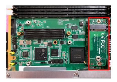
4. Screw 2 screws on M.2 carrier board (锁上螺丝, 锁固后如下)
